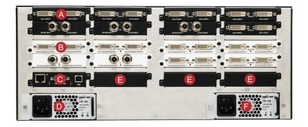
In a CORIOmatrix, slots are numbered from 1 at the top left to 16 at the bottom right. Slots 1 and 2 can only contain input modules, and slots 15 and 16 can only contain output modules. This means you can't put an audio module that has both input and output in those slots.
