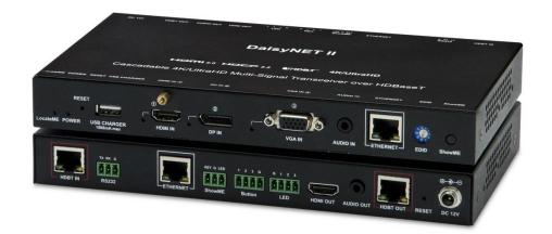
DaisyNET II is a cascadable, 4K multiformat extender for various AV signals, Ethernet and control commands. Using HDBaseT technology, DaisyNET II can distribute these signals via a CAT cable (CAT5e, CAT6A, CAT7) over a distance of up to 100 meters from device to device without quality loss or any visible latency.
