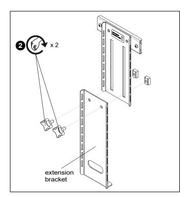
Loosen two strut nuts on back of height-adjustable bracket (A) and rotate until they are in a horizontal position. (See Figure 3)
