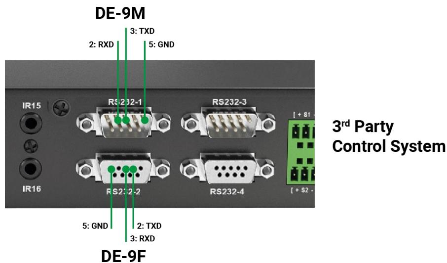
The RS-232 port on the NHD-000-CTL uses the following parameters:
